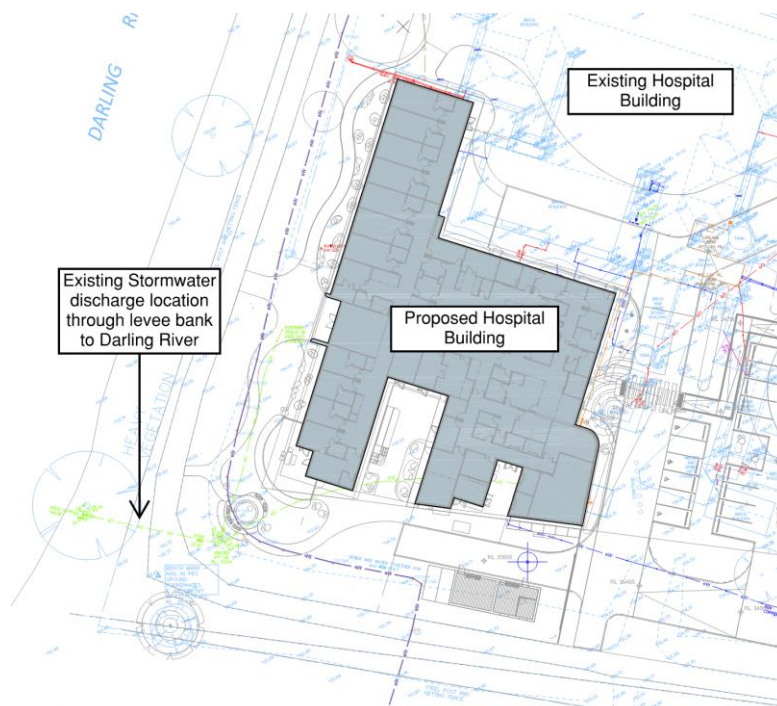
Figure 2 - Proposed site stormwater discharge point
